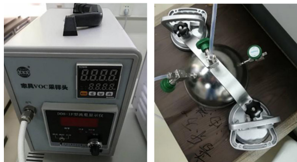
图1 木家具表面压合式采样器结构图和实物 Fig.1 The structure diagram and the authentic device of the pressed sampler for the surface of wood furniture
